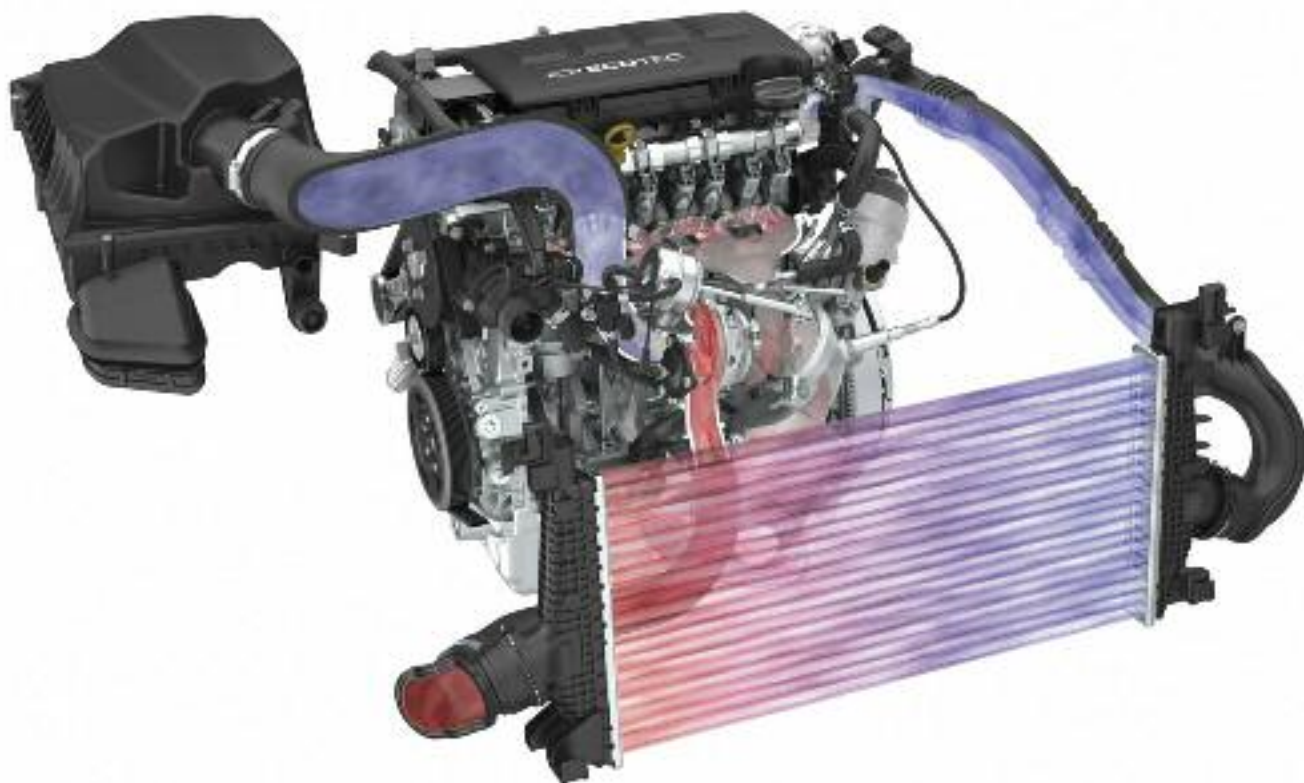
Motor de 4 cilindros “downsizing” turbo - “intercooler”- GM.
